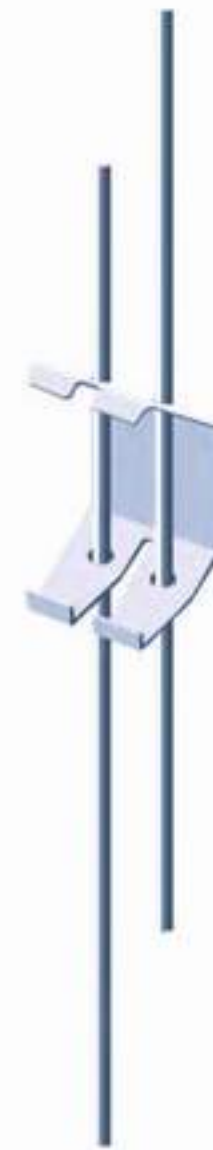
Hanging rods with adjustment clips
